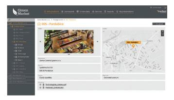
The on-line data acquisition module collects data from technologies either directly from PLCs and I/O modules, external databases, or from energy meters. It uses rich company know-how in 3rd party integration and communication using serial protocols (M-Bus, Modbus, IEC 62056-21) and APIs. The values are displayed on the portal and saved in a database. Users then have access to the entire history, anytime. Data also can be entered and edited manually, e.g. for manual energy readouts.
