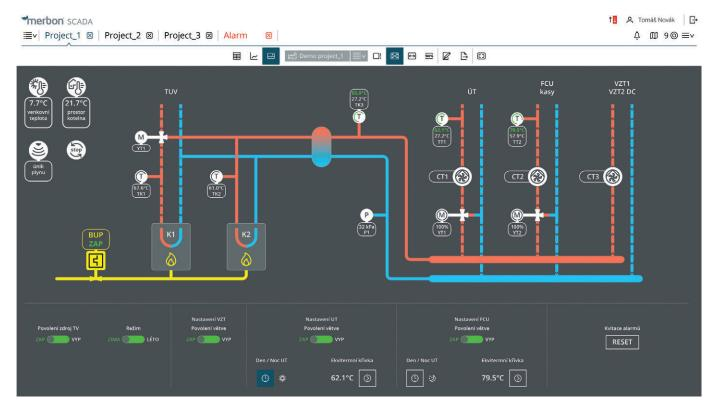
Part of the Merbon SCADA is the Merbon Alarm Server, which sends events to users according to predefined criteria depending on priority, technology unit, device location and preferred communication channel. It is thus possible, for example, to report all alarms on the computer screen during working hours and to send the user only critical alarms such as SMS requiring confirmation after the shift (according to the schedule or information from the integrated attendance system).
